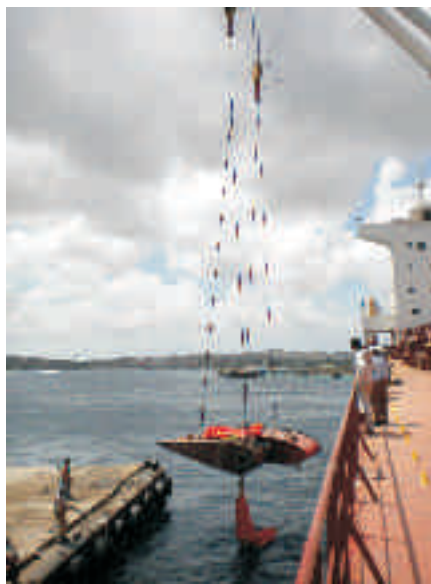
The rudder is being lifted by two of the Sophia D's four cargo cranes to lower the rudder back into the water, after the repairs on the rudder were completed in the ship yard.
